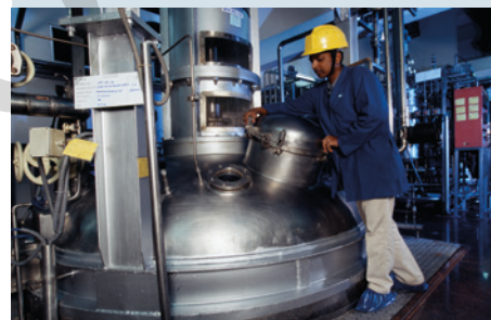
FIGURE 18.4.2 A microbe fermentation unit for the production of drugs, hormones and enzymes for medical and industrial use. It is used to ferment microbes that have been genetically engineered to produce a drug or enzyme.
